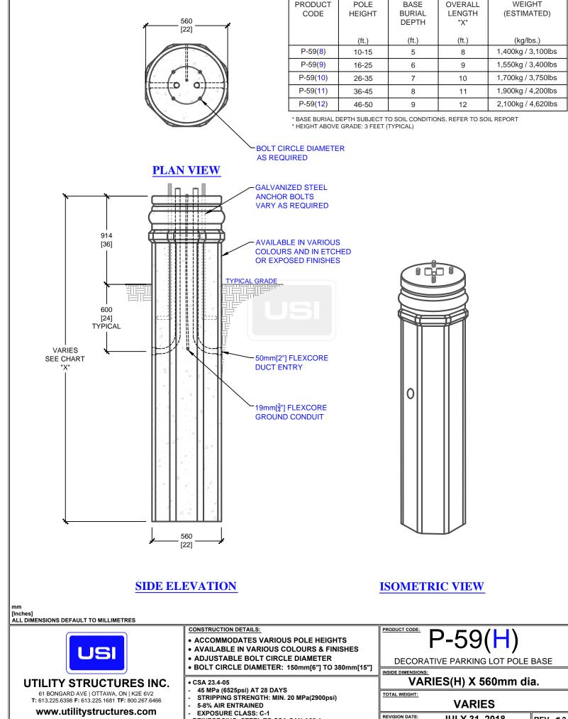
• REINFORCING: STEEL TO CSA CAN A23.1
